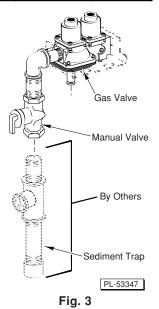
The appliance and its individual shutoff valve must be disconnected from the gas supply piping system during any pressure testing of that system at test pressures in excess of ½ psig (3.45kPa).
