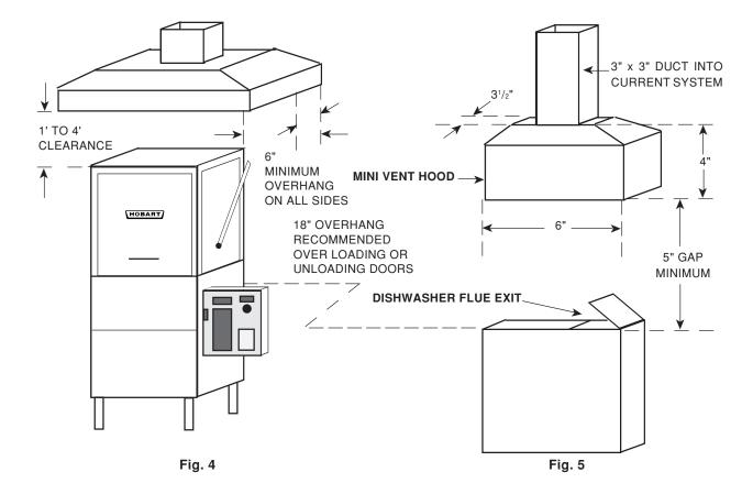
**NOTE**: Any listed and labeled factory-built commercial exhaust hood tested in accordance with UL Standard 710 by a nationally recognized testing laboratory, should be installed according to the terms of its listing and the manufacturer's installation instructions.
