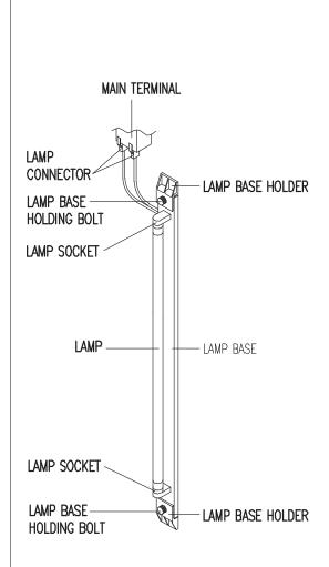
Please turn off the power before the positioning of shelves and installing a lamp.
