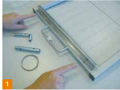
1 Remove the two wire-covers from the frame.
