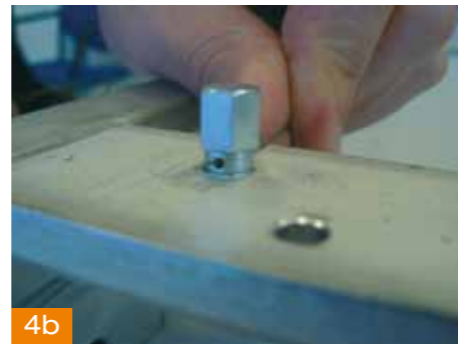
4 Screw three times the tie-rod pivots and place them with their hole parallel to the wire. See fig. 4b
