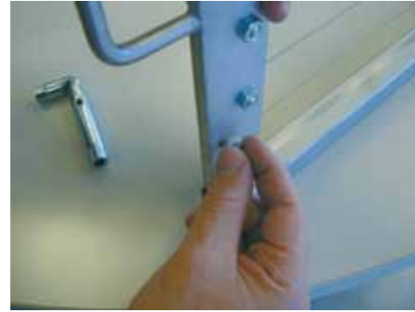
2 Slacken and unscrew the bolt which the pivots of the wire.
