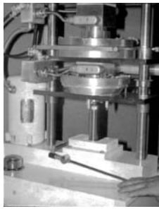
2. Press levers to form top and bottom crust.
