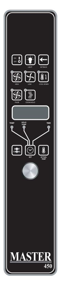
Pressing the **FAN PULSE** key will activate the lower fan speed and light its **LED**. The fan will be active for 30 seconds then off for 30 seconds, and continues this cycle.
