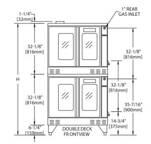
Installation Notes: Combustable Wall Clearances: Sides: 1" (25mm)
