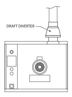
Direct venting, should be positioned on the main top and fastened with sheet metal screws provided.
