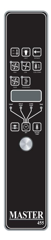
Pressing the **START/CANCEL** key will start the timing cycle. The display will count down from the Set time in minutes and seconds (solid colon) or hours and minutes (blinking colon) the minutes and seconds. When the cycle is completed, pressing this key will also cancel the "**DONE**" prompt. To cancel a timing cycle in progress, press and hold the **START/CANCEL** key for 3 seconds.
