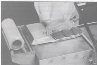
The operator places the product onto package platform inserting it between the centerfold film. Holding the product firmly with the right hand and the corner of the film with the left thumb, move the film covered product into the sealing area.
