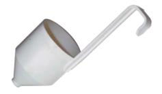
It is important when measuring viscosity that the temperature of the cup and the liquid is maintained. Heating tends to lower viscosity and even ambient temperature makes a significant difference to viscosity / flow rate. The cup needs to be dipped into the material and filled up to the top. Time how many seconds it takes until it flows through. Stop timing after the continuous flow of material from the cup has ended. This will provide the DIN/sec of that material at that temperature.
