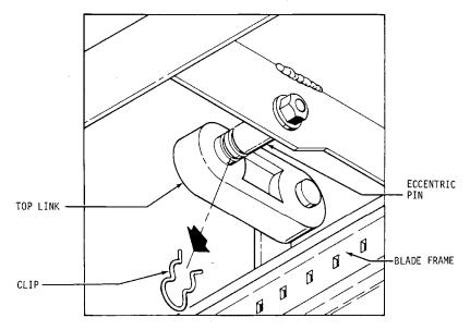
After removing the two locking cams, eyebolts and Belleville washers, (which secure the blade frame to the rocker's swing shaft), the blade frame can be removed. The eyebolts and Belleville washers can be removed by turning them counter clockwise once the cams have been removed. See illustration below.
