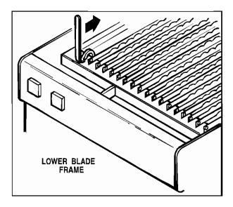
Reverse the procedure to install replacement blades. A paper clip can be used to hold the blade in position on a lower blade mount during blade installation. See the illustration below.
