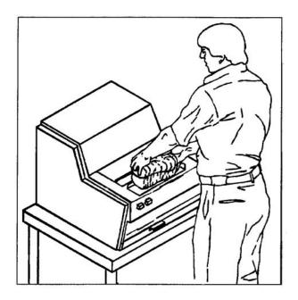
The bagging scoop is adjustable to accommodate various size loaves. To adjust, apply pressure to the bread stop and slide along scoop. See figure below.
