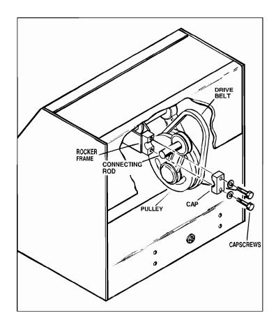
Install a new belt by reversing the removal procedure. Refer to the "Belt Tightening" section for advice on how to adjust the drive belt tension.
