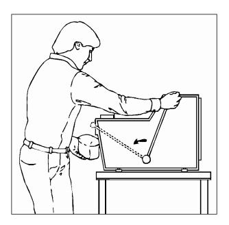
Make sure that the product does not hang over either edge of the cradle. While holding the lever completely forward (the machine will not start unless this is done), push the START button with your left hand.
