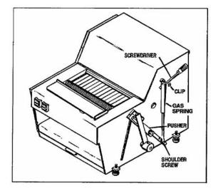
To replace the gas spring, start by re-attaching the lower end of the spring with the shoulder screw.
