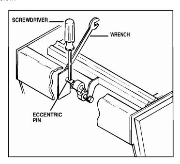
Using the small screwdriver or rod, rotate the pin to the desired position and tighten the nut to lock the pin in place. Check the frame clearance by turning the driven pulley by hand. When the adjustment is complete, replace the guards and table lip.
