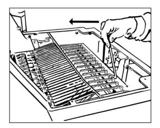
Using the same technique as used on the upper blade frame, replace the knives in the lower blade frame.
