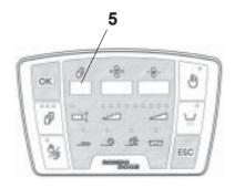
When switching on the main switch located on the base, the machine switches into the automatic-program Number 01. In the indication window of the programm number (5) appears the indication 01 and the other indication windows show the initial roller gap, the final roller gap, pre-sheeting to a width, the reduction steps and the chosen program-end.
