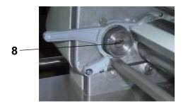
Center the catch of the machine table's driving roller in the receiver (8) in the front section of the housing
