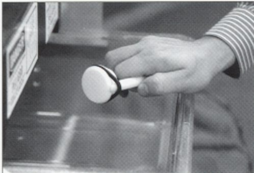
Catch tub and O ring removal tool supplied with depositor
