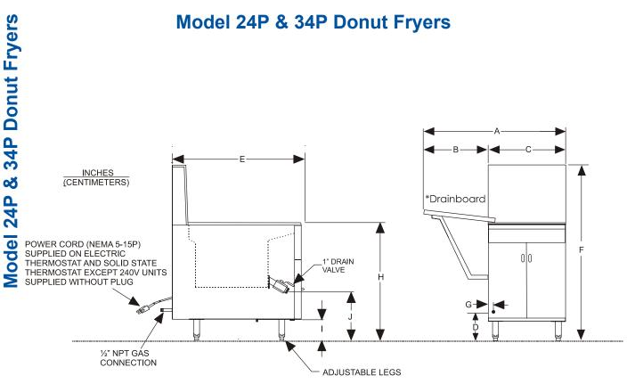
\* Drainboard is field reversible and can be used as a tank cover
