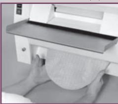
You can easily remove the Docker assembly for cleaning or when it's not needed.
